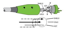
In addition to accepting balanced mic or line-level signals using an XLR connector, both channels may also accept I/4" line-level signals driven by balanced or unbalanced sources.
