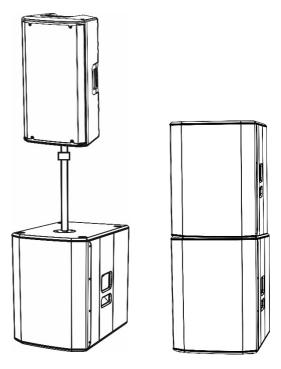
In the pictures above are shown two examples of configuration for the use of SUB 615. The matching with a speaker (like one of the OPERA or B-HYPE series) allows a perfect performance in an extended frequency range.
