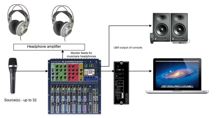
This method allows the console to receive audio from the various sources, process it using its internal DSP, distribute monitor mixes for musicians and then send each track raw to the chosen DAW for mixing later. This requires a 1 to 1 patch of each channel to a direct out of the multi digital card.
