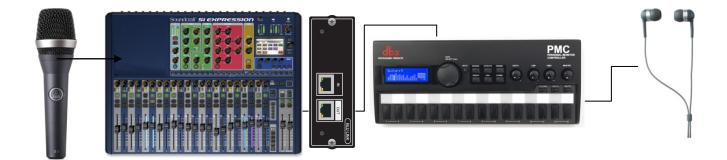
In this system we are running the inputs of the Si Expression 2 through the channel direct outputs, patching them to "BLU link 1-16". These are then being put on the network, run through a standard Cat5 cable to the dbx PMC 16 personal monitoring system. This unit then has independent level control of 16 channels of audio. This mix is individual to the musician, with the main input channel levels being controlled by the input gain controls on the console.
