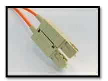
The type of connector used by the Si and Vi optical MADI cards is the 'SC' type as shown. The transceivers and fibre cable (unless otherwise specified) are the 'Multi Mode' type; offering typical distance between nodes of up to 1500m using a single run of multimode 50/125 optical fibre, 600m using 3 X 200m reels of multimode 50/125 optical fibre joined in series.
