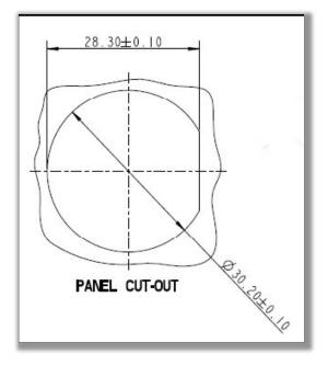
A cut-out diagram for the RZ2705-01 connector assembly is shown in the following page.
