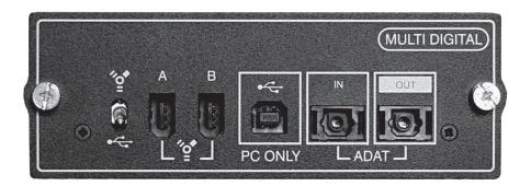
The Soundcraft® Multi Digital card offers digital audio connection between an Si Series console\* and Apple® Mac® enabled with Firewire (1394), or PC enabled with a USB or Firewire port. Audio capability across the Firewire or USB link is 32 channels in and 32 channels out at 48KHz. In addition to the Firewire/USB ports, the Multi Digital card provides 8 further channels of ADAT in and out at 48KHz.
