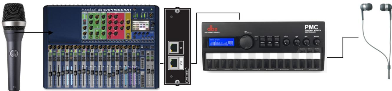
In this system we are running the inputs of the Si Expression 2 through the channel direct outputs, patching them to “BLU link 1-16”. These are then being put on the network, run through a standard Cat5 cable to the dbx PMC 16 personal monitoring system. This unit then has independent level control of 16 channels of audio. This mix is individual to the musician, with the main input channel levels being controlled by the input gain controls on the console.
