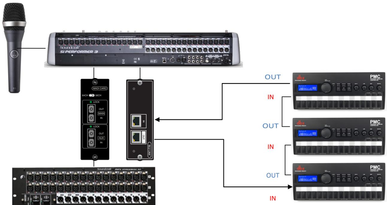
When BLU link is used with a Soundcraft Si Performer, you can run a stagebox on one option slot using MADI, and a BLU-Si card connected to the PMCs through BLU link in the second slot. This would allow for remote I/O and a personal monitoring system on a larger show where the console is located further from the stage.
