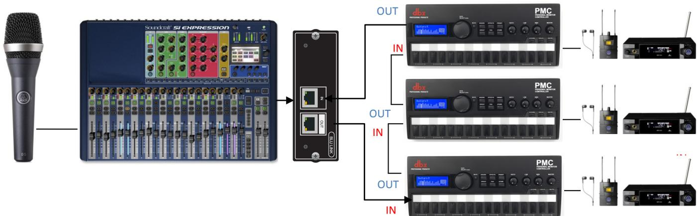
The above diagram shows 3 personal monitoring units receiving all 32 channels being sent from the console, from which each PMC may select its own 16 channels for a personalised mix. The stereo line or XLR outputs of the PMC can also be sent to a wireless in-ear transmitter system for freedom of movement.
