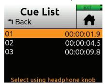
2. Tap Move and rotate the HP encoder to adjust the selection in 0.1 second increments.
