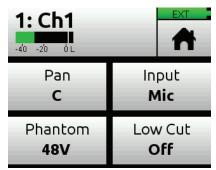
There, you'll be able to select the channel input source, whether you'd like to send the audio to the Left, Center or Right of the mix bus, select Phantom power (for condenser microphones and active DIs), and select a Low Cut Filter.
