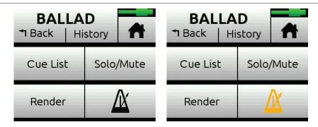
① The Metronome button will be disabled (appearing grayed out but with an orange icon) whenever Click is assigned as a track's input source.
