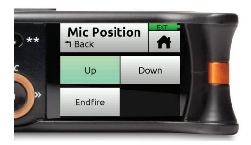
Select from Up, Down, or Endfire. It is essential that this setting is correct to ensure the sound space is mapped correctly.
