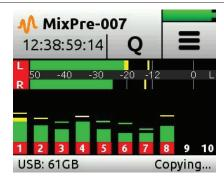
rianlge Do not remove the USB thumbdrive from the recorder when Copying is in progress.
