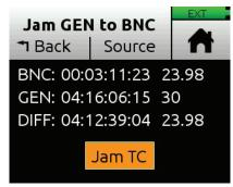
The screen displays the internal and external timecode, and the difference (Diff) between the two values.
