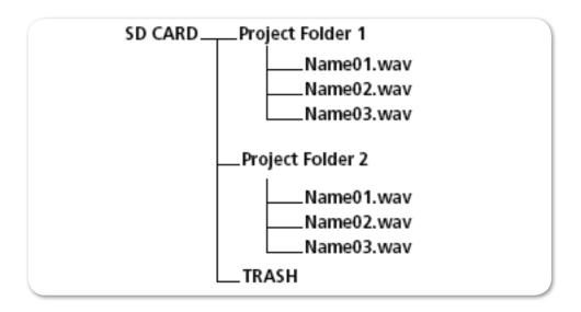
Only one project is active at any one time. If you choose not to create a project, the MixPre-10T automatically creates one with the current date as its name. The project folder contains all files recorded during the time that project is active. Rerecorded files are always placed in the same project folder as the source file. Project files are sorted by creation date. All active project's files can be viewed in the File List.
