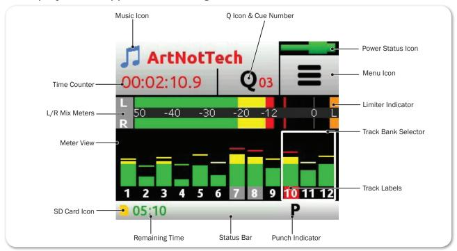
① The sample image shows the Home screen on a MixPre-3, as indicated by the Track Bank Selector (white box) being around only three meters. This appears differently on the MixPre-6 and MixPre-10T.
