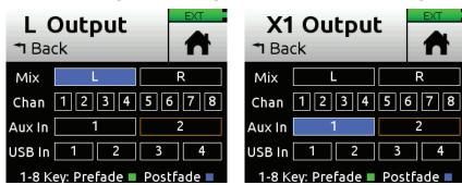
In addition, if you choose to send the channels to outputs, you can select either pre-fade (Channel knob has no effect) or post-fade (Channel knob controls level).
