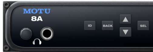
Figure 6-2: The volume knob is a push-button digital rotary encoder.
