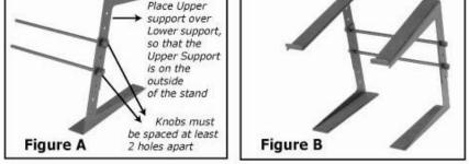
1. Take one of the upper supports and place it over one of the lower supports (see figure A). Align the upper support holes with the lower support mounting holes to obtain the desired height. Place one knob at a time through the mounting holes (must be spaced at least 2 holes apart). Take a stabilizer bar and screw the top knob into the end of the stabilizer bar. Repeat with bottom knob.
