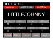
The first parameters you encounter are the ones we considered most useful, and they've been selected from different menus. But you can edit any of the device's parameters by pressing the Menu button (D5), which will activate the scroll menu. From here you can access every menu in the selected device.
