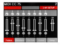
Move the faders and their values will update in the display as they move. Where controls are assigned to send a standard MIDI Controller message, pressing the **TOGGLE/VIEW** button (K) will display the Controller number assignments. Pressing the **TOGGLE/MUTE** button (H) will mute the MIDI output of the faders, so you can position them where you want them. Press again to unmute.
