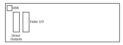
....or on 2 x 25-way D-type connectors, each handling 8 audio paths:
