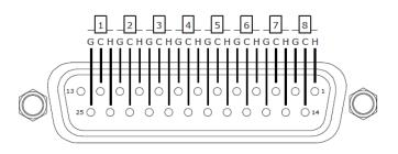
Looking at the fader pack from the rear, the connector on the  ${\bf right}$  is for channels 1 – 8.
