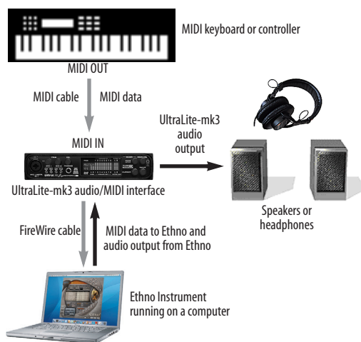
Figure 4-2: An example setup for stand-alone operation using a MOTU UltraLite-mk3 audio interface. In this example, the UltraLite-mk3 is also handling MIDI data transmission from the keyboard controller to the computer and Ethno Instrument.
