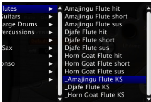
Figure 7-4: Keyswitch (KS) presets. In this example, the KS preset (selected) provides three layers made up of the Amajingu Flute presets above (hit, short and sustain).
