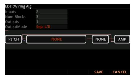
In the Wiring Alg Editor, each function block has three editable parameters: number of inputs, number of outputs, and block size. (The Output Mode parameter applies to the entire algorithm.)
