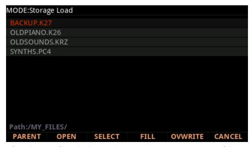
After selecting a file to load, press the OPEN, FILL or OVWRITE soft button to continue
