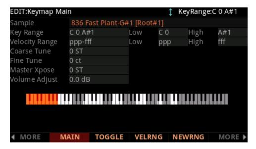
If you want to select a different sample, use the cursor buttons to select the Sample parameter. Use the Alpha Wheel to select a sample. Press the **EDIT** button once more, and you'll enter the Sample Editor. The sample will play through the effects of the current program. The name of stereo samples end with an **S**. To use a stereo sample, the <u>Stereo</u> parameter must be set to On in the Program Editor, and two Keymaps must be selected, see The KEYMAP Page on page 3-44.
