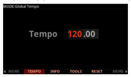
Set the Tempo parameter with the Previous/Next buttons, the Alpha Wheel, or alphanumeric entry. You can also set the system tempo by using the TEMPO section of the front panel. Press the TAP button a few times at the desired rate, or use the TEMPO knob.
