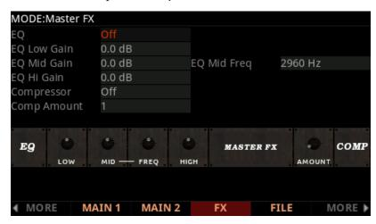
When the Compressor is set to On, use the Comp Amount parameter to set the compression amount between 1 (least compressed) and 11 (most compressed).
