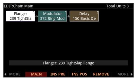
At the top right of the display is the number of FX units used by the currently selected effect-box, and by the Chain as a whole. There are a total of 32 units available for all of the Chains that are currently loaded by programs and any active Aux overrides from Multi Mode.
