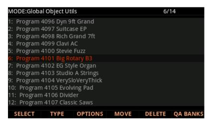
Use the navigation buttons to highlight the object that you wish to move or delete, then press the **SELECT** soft button to select the object. Selected objects are marked with an asterisk, and multiple objects can be selected at the same time.
