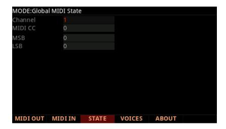
For example, if a channel is not making any sound, you can check the values for MIDI CC 7 (Volume) and MIDI CC 11 (Expression). Use the cursor buttons to select the Channel or MIDI CC fields, then use the alpha wheel or previous/next buttons to select the desired Channel and MIDI CC to view.
