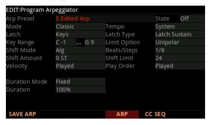
In Multi Mode, the Arpeggiator works the same as in Program Mode, except there is one arpeggiator per Zone. The Arpeggiator in each Zone can each have different settings, and they can be played at the same time. Also, in Multi Mode the Arpeggiator page does not have the Tempo parameter, instead the **Tempo** parameter on the Multi Common page should be used.
