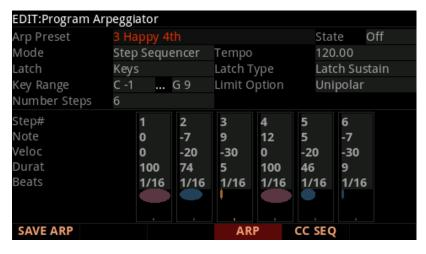
Select a parameter using the up/down navigation buttons. To change steps, select the Step# parameter, then press the left or right navigation buttons.
