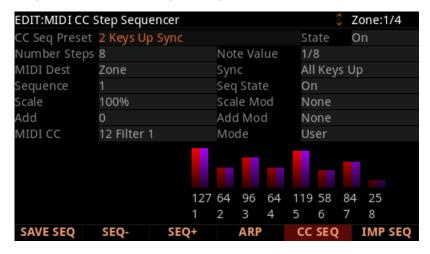
In Multi Mode, the CC Sequencer works the same as in Program Mode, except there is one CC Sequencer per Zone. The CC Sequencer in each Zone can each have different settings, and they can be played at the same time.
