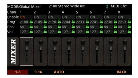
The Mixer page allows you to view and control the current state of the K2088/61's 16 MIDI channels. The currently selected Channel and Program are displayed in the top line. Press the **1-8** or **9-16** soft button to view channels 1-8 or 9-16.
