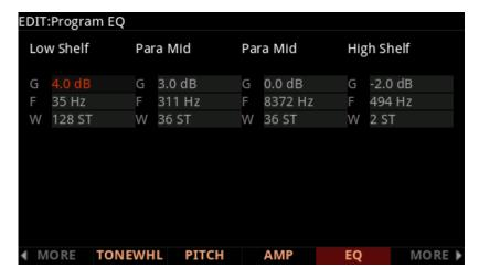
Each EQ section has **Gain** (**G**), **Frequency** (**F**), and **Width** (**W**) controls. **Frequency** controls the center frequency of the band. **Width** controls the bandwidth. **Gain** controls the amount of boost or cut.
